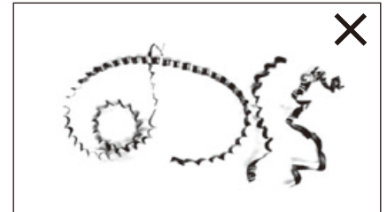
Continuously coiled long chips
