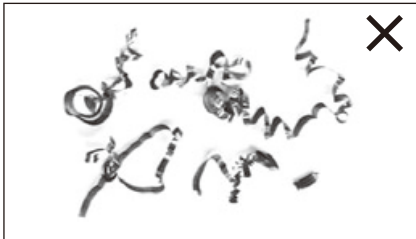
Apple-peel-like chips (Without curling)
