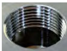
THREADMILLING ETTL25M017W25.0F026R02-PT, TL25SEIR11BSPT
