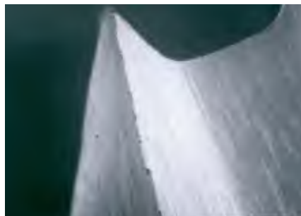
Surface of a conventional fluteless tap
