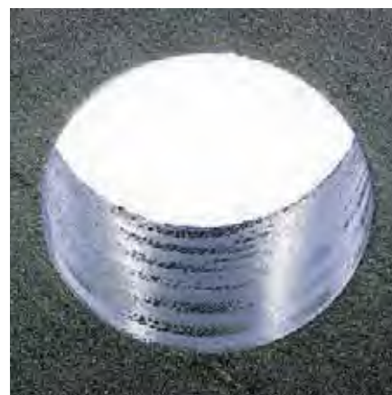
Hole D = 6.35 mm Unidirectional CFRP with optimal machining quality
