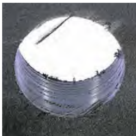
Hole D = 6.35 mm With fibre projection on cover coating and delamination
