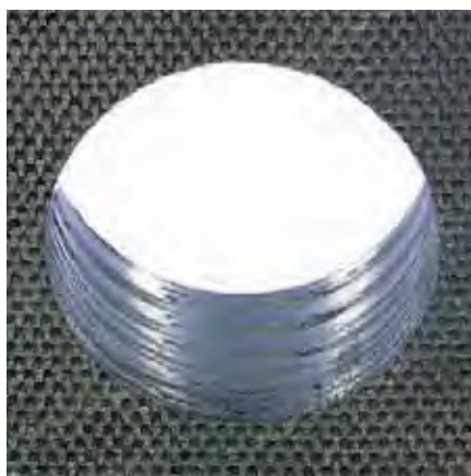
Hole D = 6.35 mm CFRP with fabric layer, optimal machining quality
